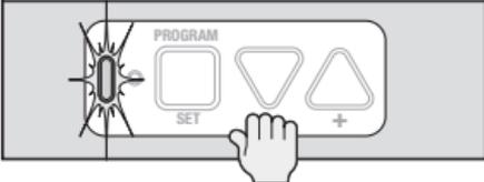
**3** Press and hold the **down arrow button (-)** until garage door is fully closed on floor, then release.
