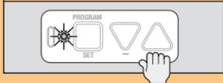
**7** Press and hold the **up arrow button (+)** until door is fully open, then release. Watch carriage as it approaches the powerhead to avoid contact with powerhead.
