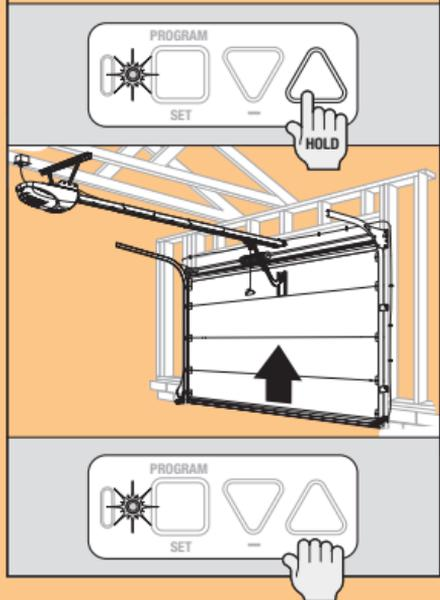
**8** Press and release the **Program Set button** (both LEDs flash blue and go off).
