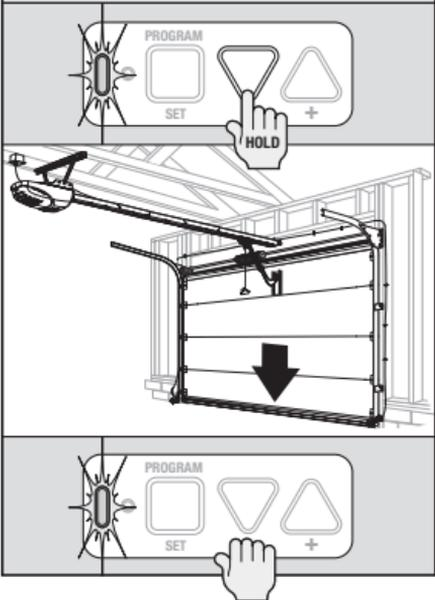
**4** Press and release the **Program Set button** (both LEDs flash blue and go off).
