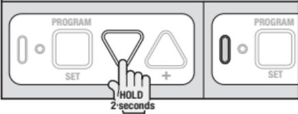
**2** Release **down arrow button (-)** and the long LED will begin flashing.
