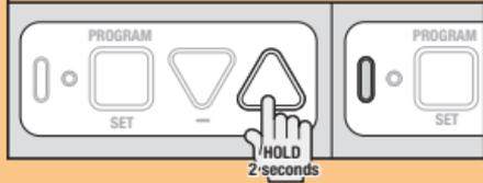
**6** Release **up arrow button (+)** and the round LED will begin flashing.
